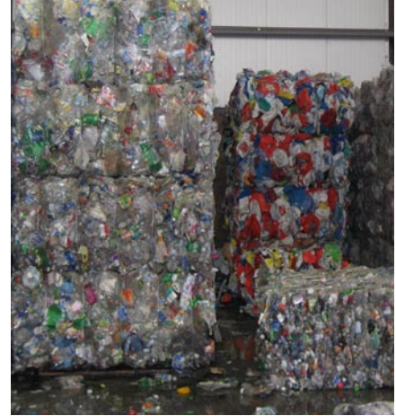
Recycled material separated and compacted; ready for shipment at the Sunset Scavenger Recycling Company, which recycles the solid waste collected at SFO.
